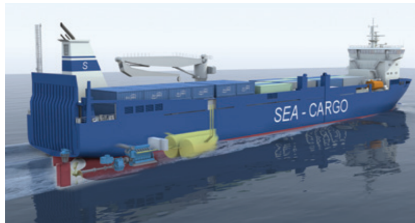
Illustration newbuilding Hull 357 of Sea-Cargo, propelled by LNG With kind permission of Sea-Cargo
